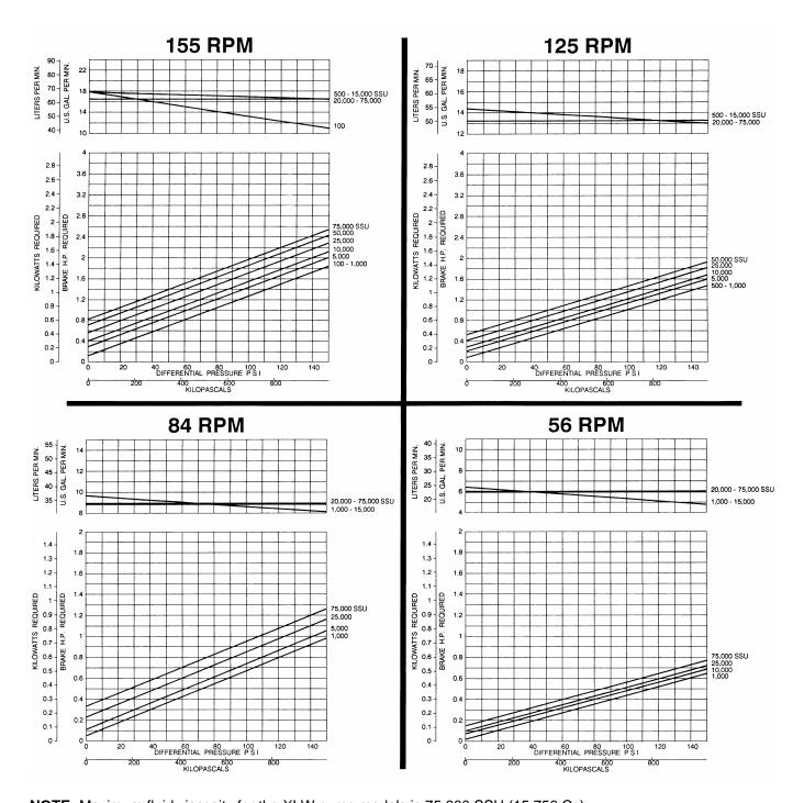
NOTE: Maximum fluid viscosity for the XLW pump models is 75,000 SSU (15,750 Cs).
