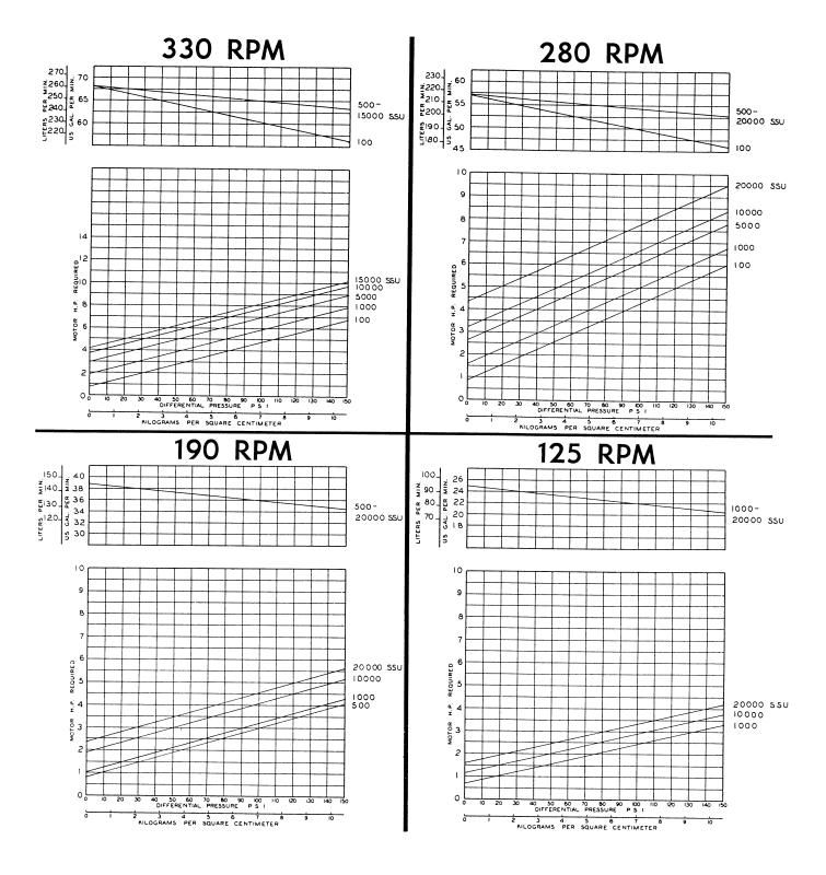
Actual capacities are dependent upon the vapor pressure of the liquid, the suction lift and the inlet line losses of the system. Blackmer characteristic curves are normally based upon a inlet condition of 5" to 8" Hg. vacuum and zero liquid vapor pressure.
