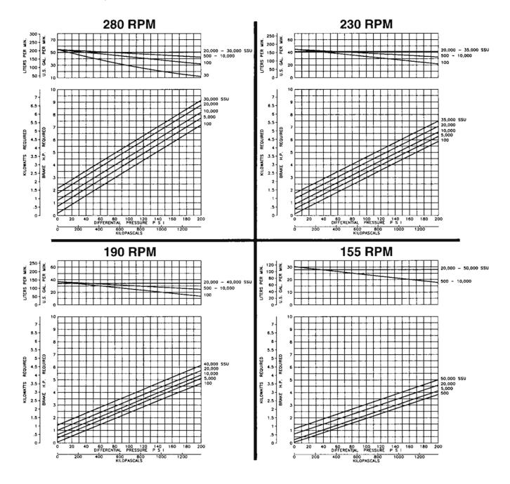
**NOTE:** Blackmer Characteristic Curves are based on Brake Horsepower (BHp). To determine Motor Horsepower, drive train inefficiencies must be added to the BHp.
