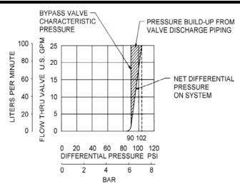
For example, the BV0.75 and BV1 bypass valves have a characteristic pressure when set at 90 psi (6.21 bar) as shown on the following curve. If the friction loss through the bypass valve, discharge pipe and fittings (pipe, elbows, tees, shut-off valve, check valve, etc.) is 12 psi (.84 bar) at 100 gpm (379 lpm) flow rate, then the actual differential pressure in the system will rise under bypass conditions, as illustrated on the curve.
