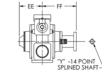
Splined Shaft Hydraulic Drive Option
