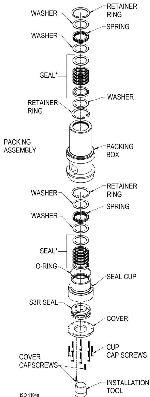
**Fig. 13a – Packing Box Assembly**
