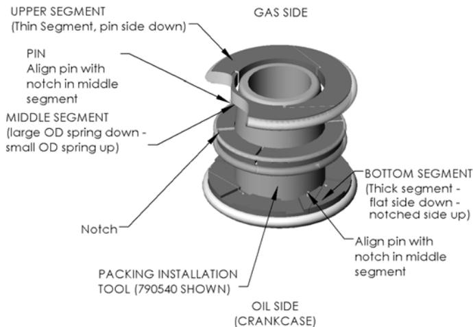
Figure 13c - S3R Oil Seal Installation
