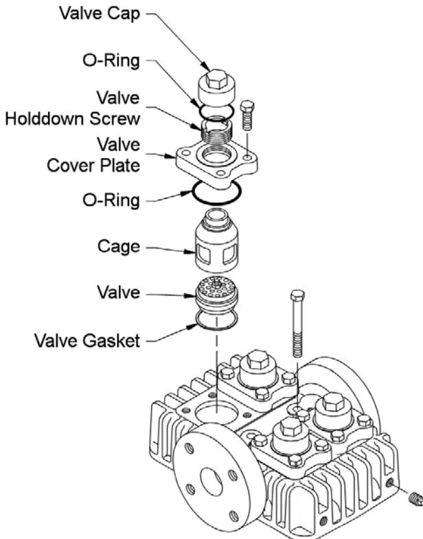
**Fig. 9 – Typical Head Assembly**
