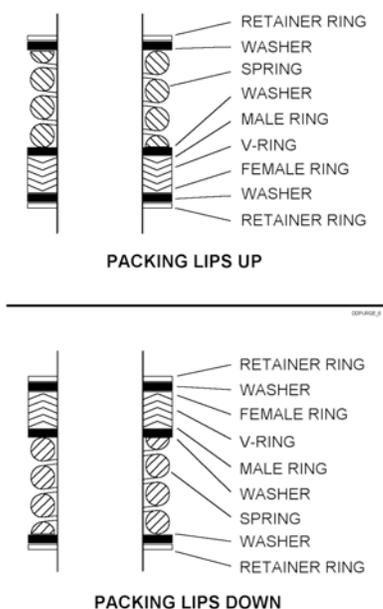
**Fig. 11 – Seal Component Orientation**
