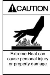
Discharge piping surface temperatures may be hot during operation (over 158°F, 70°C). Temperatures should be monitored and adequate warnings posted
