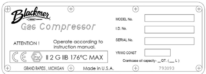
The basic size and type of the compressor is indicated by "Model No." A suffix letter is used to indicate the version.
