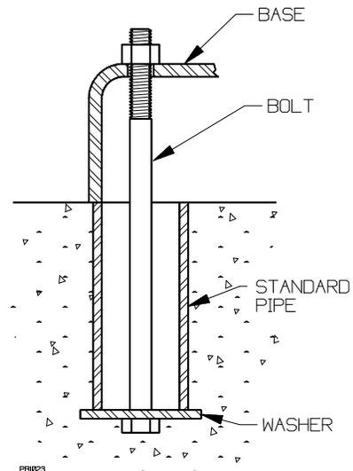
Figure 2 - Anchor Bolt
