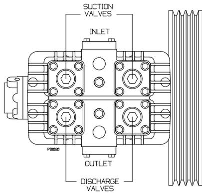
**Fig. 8 – Valve Locations, Single-Stage Models**
