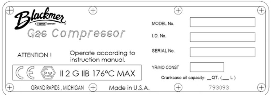
**Figure 2 - Compressor Nameplate**
