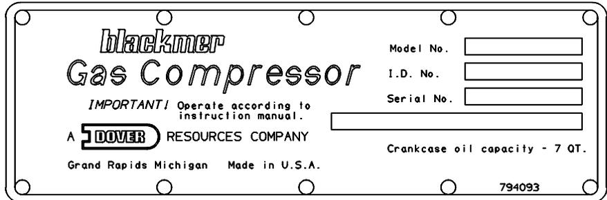
Model No. Indicates the basic size and type of the compressor.
