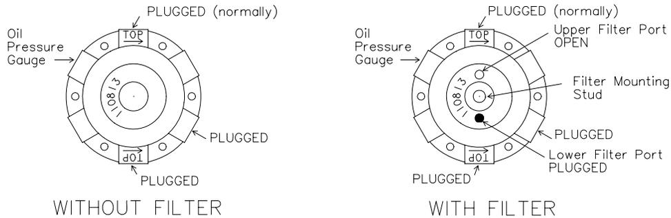
9. Verify that the proper plugs are installed in the oil pump cover per the above sketches.
