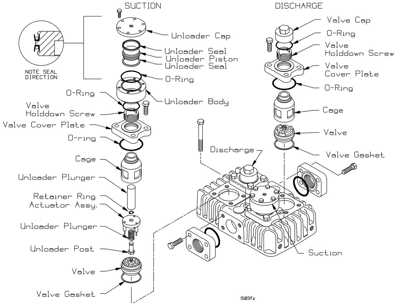
Typical Head Assembly (with Suction Valve Unloaders).
