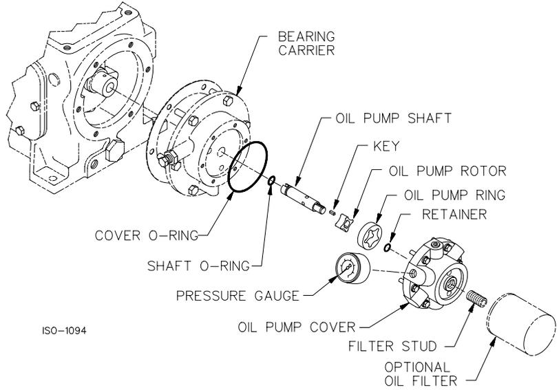
5. Place the oil pump ring over the rotor. Place the cover O-ring into the bearing carrier (do **not** place it on the oil pump cover).
