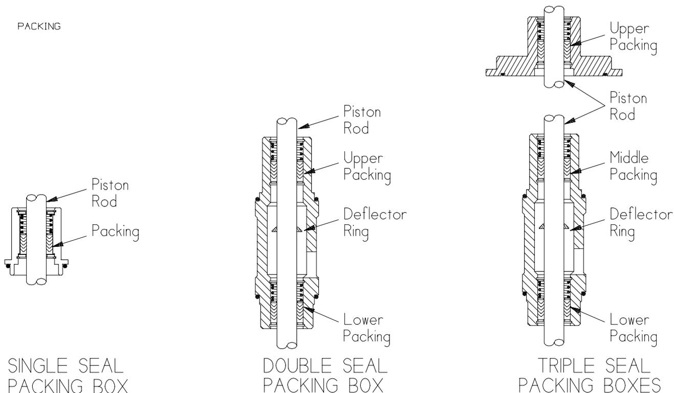
Compressor ID# identifies the packing orientation.
