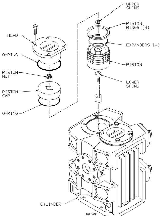
Figure 8 - Cylinder and Piston
