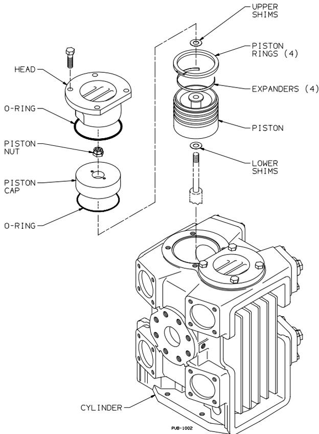
**Figure 11 - Cylinder and Piston**
