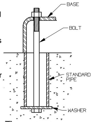
**Figure 3 - Anchor Bolt**
