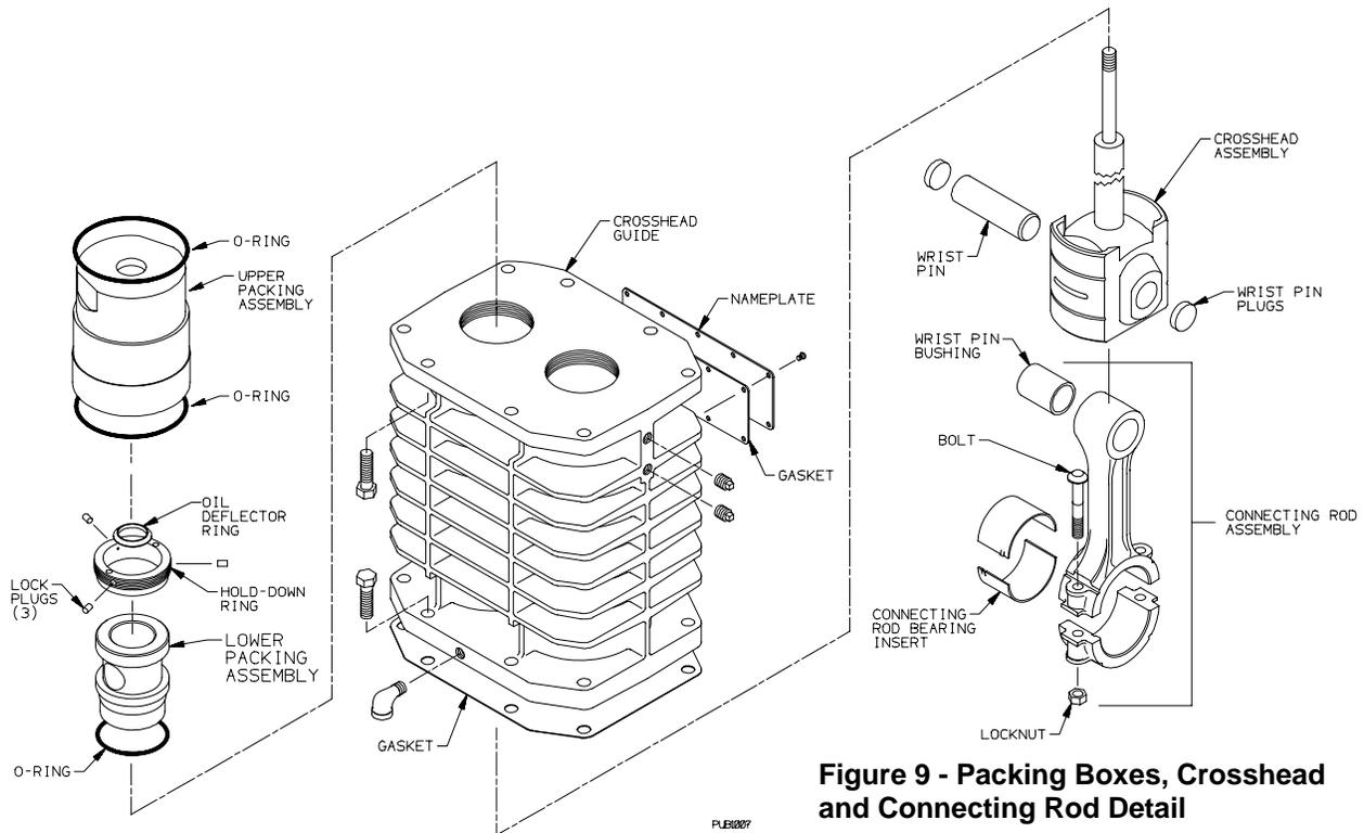
**Figure 9 - Packing Boxes, Crosshead and Connecting Rod Detail**
