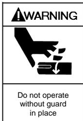
**Failure to adjust guards covering all rotating part, allowing only a safe gap, can cause personal injury or death**
