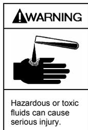
Containment can failure will permit fluid leakage and can cause serious injury.
