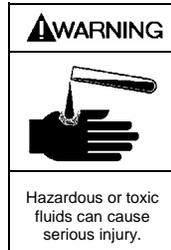
**IF PUMPING HAZARDOUS OR TOXIC FLUIDS, SYSTEM MUST BE FLUSHED AND DECONTAMINATED, INSIDE AND OUT, PRIOR TO PERFORMING SERVICE OR MAINTENANCE**
