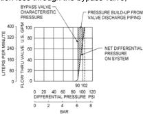
For more information on sizing and friction loss, refer to the Blackmer Liquefied Gas Handbook - Bulletin 500-001 (or Bulletin 33 for other liquids) for pipe friction tables.
