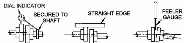
Figure 5 – Coupling Alignment
