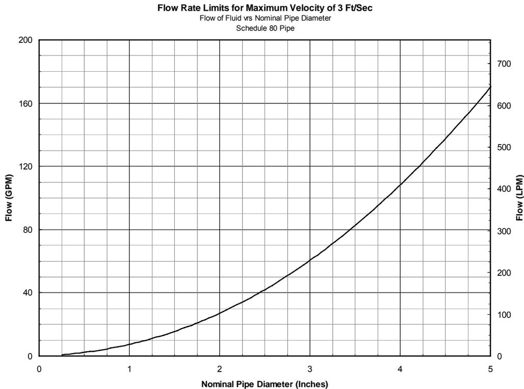
Figure 5. Flow Limits for Various Inlet Pipe Sizes for a Velocity of 3 Ft/Sec
