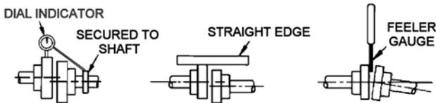
Figure 3 – Alignment Check
