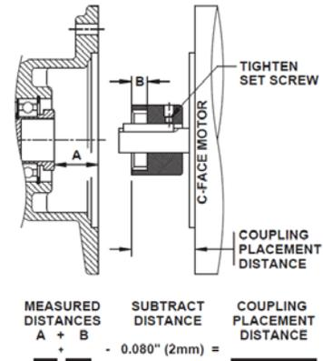
“J” Style NEMA Motor Coupling Installation
