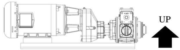
Figure 10 - Standard Gearbox Orientation
