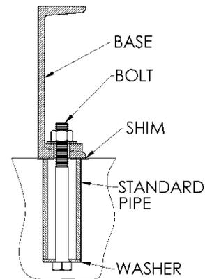
Figure 2 - Pipe Type Anchor Bolt Box
