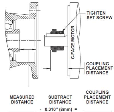
“M” Style NEMA Motor Coupling Installation
