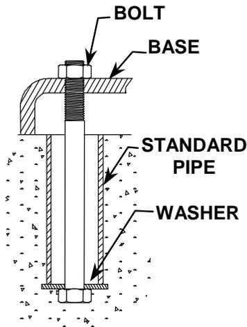
Figure 4 – Pipe Type Anchor Bolt
