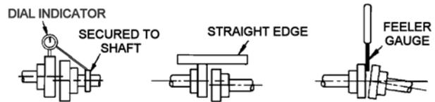
Figure 5 – Coupling Alignment
