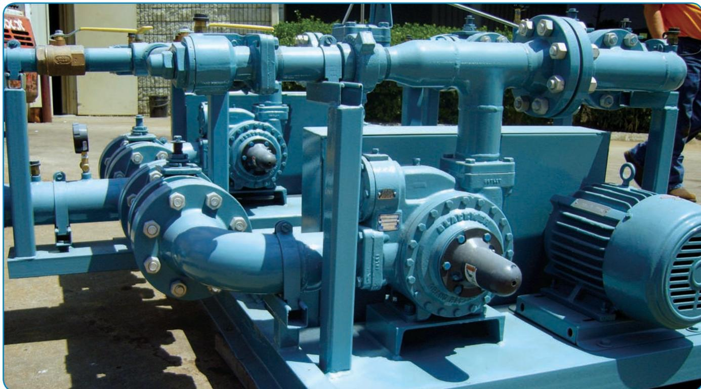
Ely Energy is a worldwide leader in large-scale SNG and LPG vaporization systems. One of the company's newest vaporization systems (pictured) features Blackmer LGL Sliding Vane Pumps.
