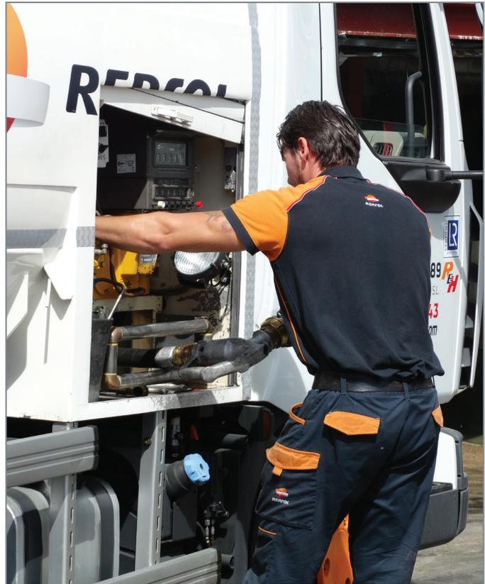
Heating oil and diesel fuel deliveries must be completed in a timely, safe and reliable fashion. By equipping all of its delivery trucks with TX Series Sliding Vane Pumps from Blackmer®, Reques e Hijos is able to satisfy the demands of these critical operations, especially in the cold winter months when service interruptions cannot be tolerated.
