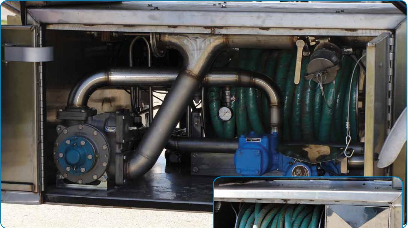
With the help of truck and transport builder Liquid Haulers Maintenance (LHM), Moline, MI, USA, Brenner Oil is able to deliver bulk quantities of DEF with the help of a Blackmer® STX3-DEF sliding vane pump.
