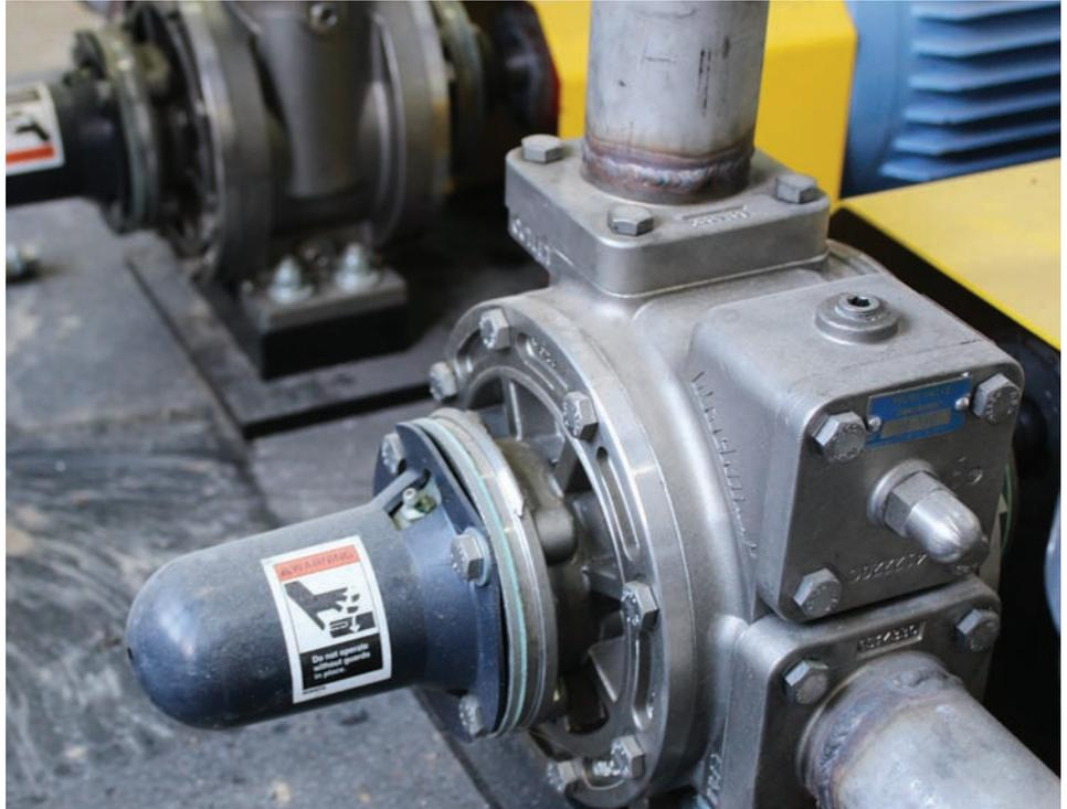
Pumps used during the DEF production and loading/unloading process must be compatible with DEF’s unique characteristics. This is why Brenntag North America relies on STX-DEF Series Sliding Vane Pumps from Blackmer®.
