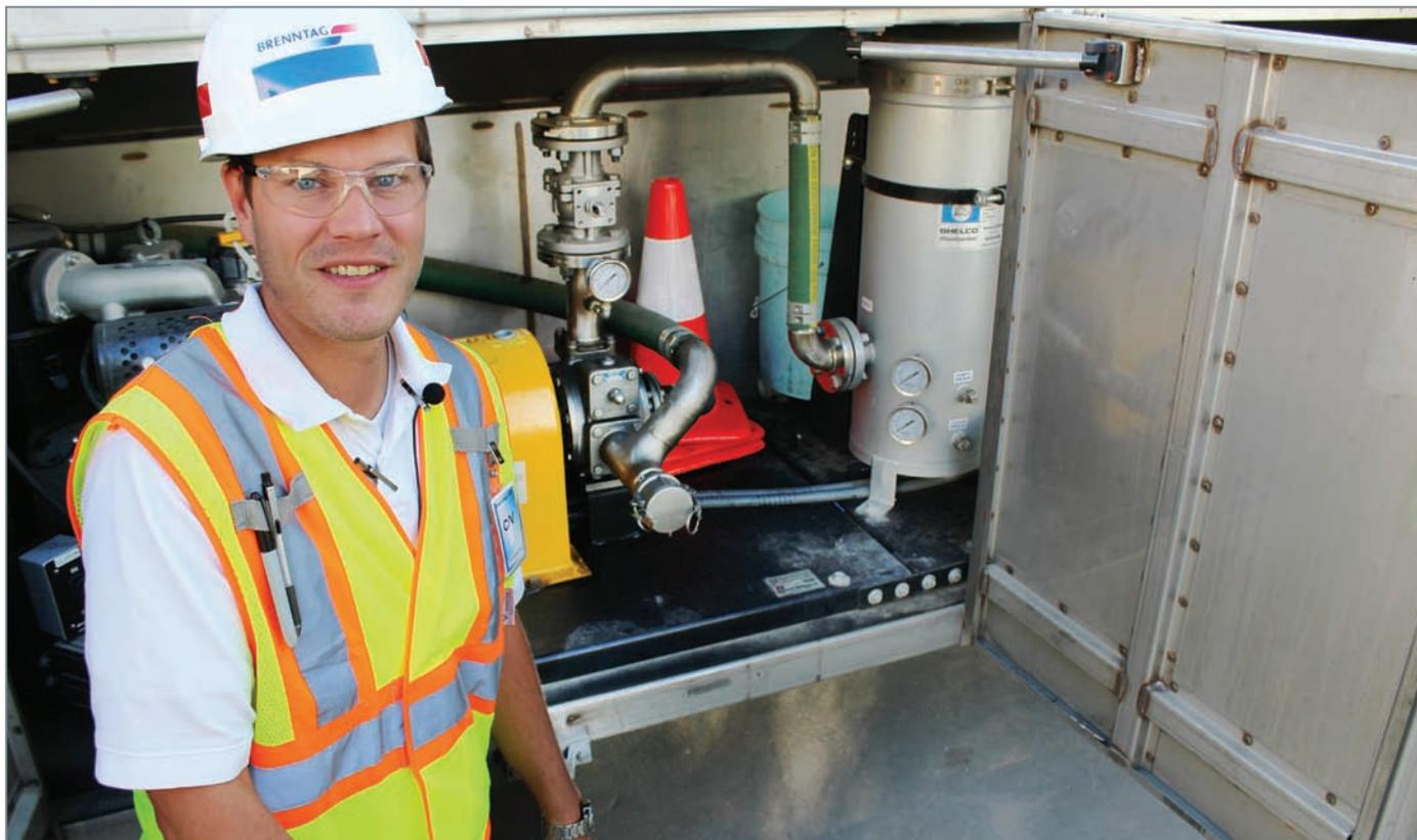
Delivering Diesel Exhaust Fluid (DEF) can be challenging. This is something that DEF Mechanical Engineer Matthew Sparrow, and the company he works for, Brenntag North America, knows all too well. So in order to ensure the safe and efficient delivery of its DEF, Brenntag North America utilizes STX-DEF Series Sliding Vane Pumps from Blackmer®.
