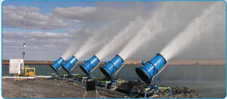
Due to new regulations, Australian mine operators can no longer discharge water into nearby waterways. Today, the most efficient and effective way to eliminate this water is through an evaporation process.
