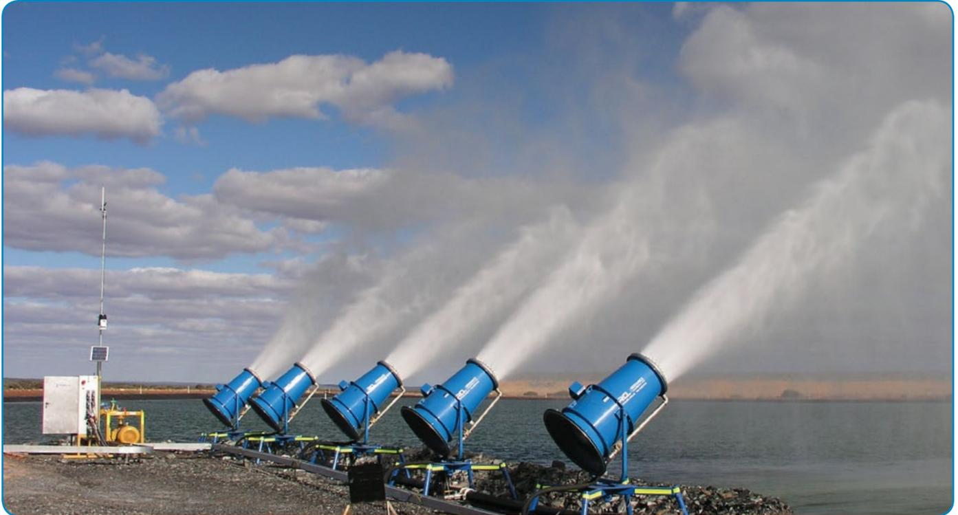
Due to new regulations, Australian mine operators can no longer discharge water into nearby waterways. Today, the most efficient and effective way to eliminate this water is through an evaporation process.
