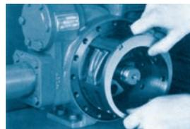
Easily replaceable liner restores efficiency.
