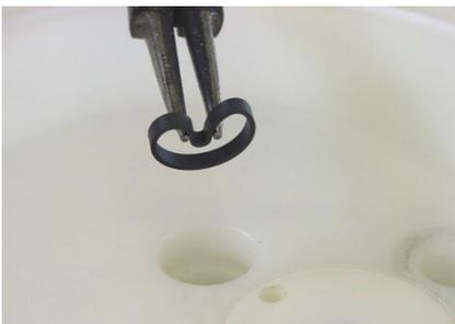
To assemble new piston rings [22] (pump sizes E 15 - E 50 only), carefully shape them like kidneys with snap ring pliers and insert the rings into the grooves in the center housing [4] (figure 15.1); completely press the rings into the grooves smoothly using some round tool.
