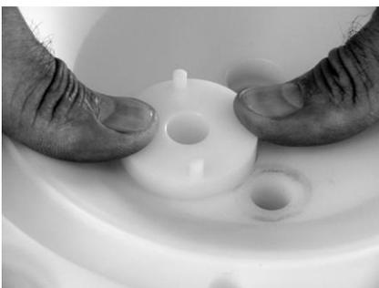
Push out the air-valve housing with the mounting tool turned around.
