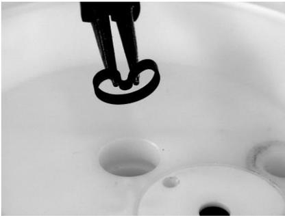
To install a new piston ring [17], carefully shape it like a kidney (see picture on the left) and with locking ring pliers and insert the ring into the groove in the center block [16]; completely press the rings into the grooves smoothly using some round tool.
