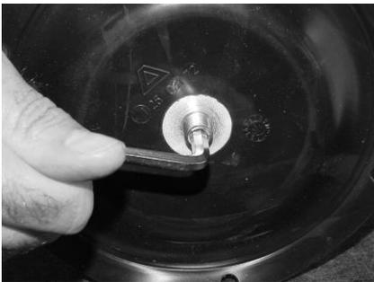
Screw out the set screws, shaft [13a].
