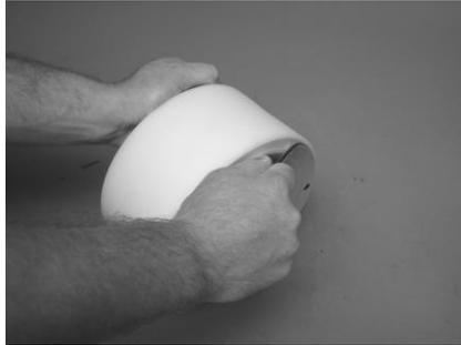
Screw one diaphragm [14] counterclockwise off the shaft [13].
