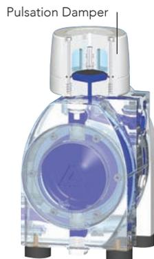
An optional Pulsation Damper buffers the periodic pressure decreases, resulting in a virtually uniform flow. It screws directly to the delivery side of the pump, eliminating the need for additional piping between the pump and the damper.
