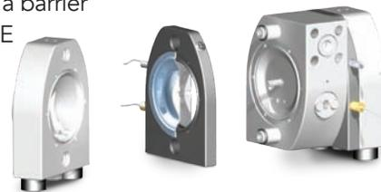
The Internal Drain System consists of a bypass system in the side housings that can be activated either through hand-operated valves or pneumatically, which allows the pump and piping to be drained without having to be disconnected. This capability also reduces the amount of cleaning agent and solvent that is needed, which also greatly reduces environmental pollution. All of these capabilities make possible the recovery of high value liquids.
