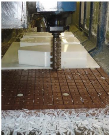
The pump's solid-body PE or PTFE block construction increases its strength and operational life cycle while eliminating many maintenance concerns. The pump's body and other components are CNC-machined rather than, as is the case with many competitive models, injection-molded.
