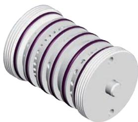
With its PERSWING P® Air Valve Almatec enables its E-Series pumps to achieve superior efficiency in flow rate and air consumption, which translates into lower energy costs. The highly accurate reversal of the main piston, which has only two moving parts, results in low noise levels, less required maintenance, and stall-free operation.
