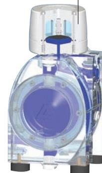
An optional Pulsation Damper buffers the periodic pressure decreases, resulting in a virtually uniform flow. It screws directly to the delivery side of the pump, eliminating the need for additional piping between the pump and the damper.
