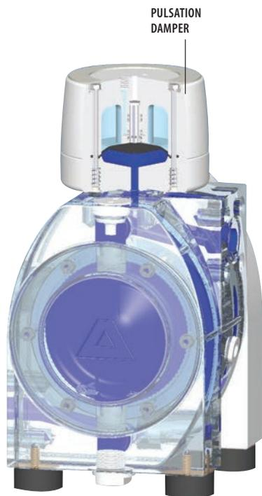
Due to their design, pumps with oscillating action produce a pulsating flow. Although the double-acting design of the E-Series and the direct pneumatic drive have already greatly reduced the pulsation, a pulsation damper must still be installed on the delivery side in order to obtain a virtually uniform flow.
