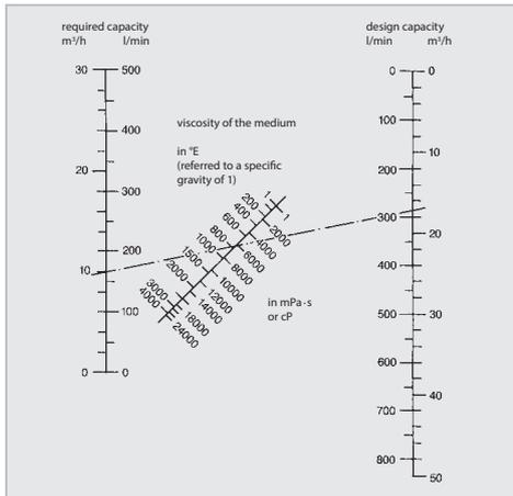
The capacity specified in the pump performance charts generally refers to water (1 mPa·s). The value must be reduced correspondingly when pumping media with higher viscosity. The design capacity can be read off directly from the graph and the corresponding pump size selected.
