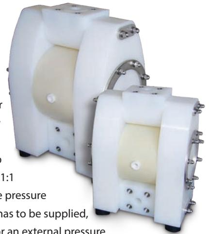
Users who need a high discharge pressure of 15 bar (218 psig) — no matter whether it is a AHD pump with internal pressure transmission or an AHS pump that achieves the discharge pressure by means of an external booster — can do so safely because the pump is designed for such pressure ranges and does not have to be held together by external reinforcements.
