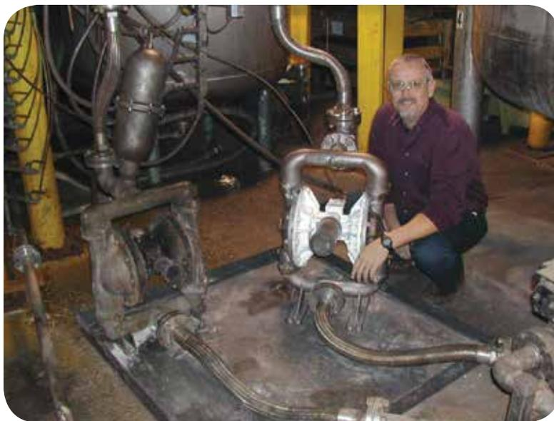
Scott Schmidt, president of Catalyst Refiners' catalyst operations, next to All-Flo's newest air-operated diaphragm pump. Catalyst Refiners' silver-based catalyst recycling operations are powered throughout the facility by diaphragm pumps.
