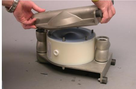
Remove side housing [1] and suction/discharge ports [2].
