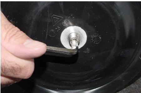
Screw out the set screws, shaft [13a].
